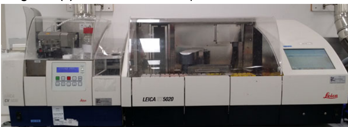
Figure 5: Automated stainer (Leica ST 5020) on right and automated coverslipper (Leica CV 5030) on left
